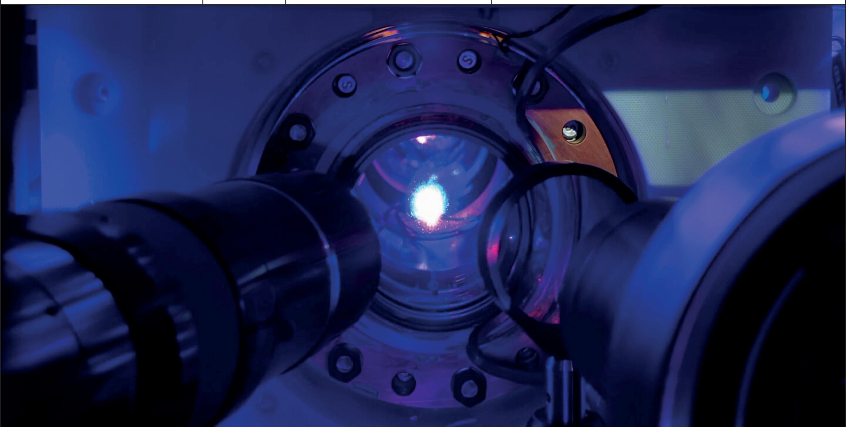
By shining an ultra-precise laser on strontium atoms, researchers have created the world's most accurate atomic clock. The laser's frequency is fine-tuned to make an electron in the strontium atom jump between its energy levels, and the clock is synchronized to this frequency. It then measures time to within a billionth of a billionth of a second.
