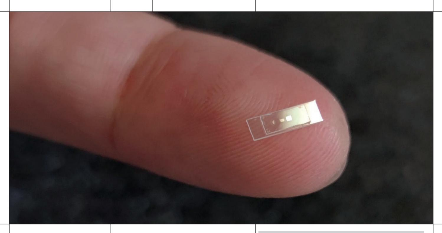
This electronic component weighs 16 micrograms—just enough to be visible to the naked eye. By cooling it, a team successfully placed it in two states simultaneously: a spring both stretched and compressed, mirroring Schrödinger's cat being both dead and alive.
