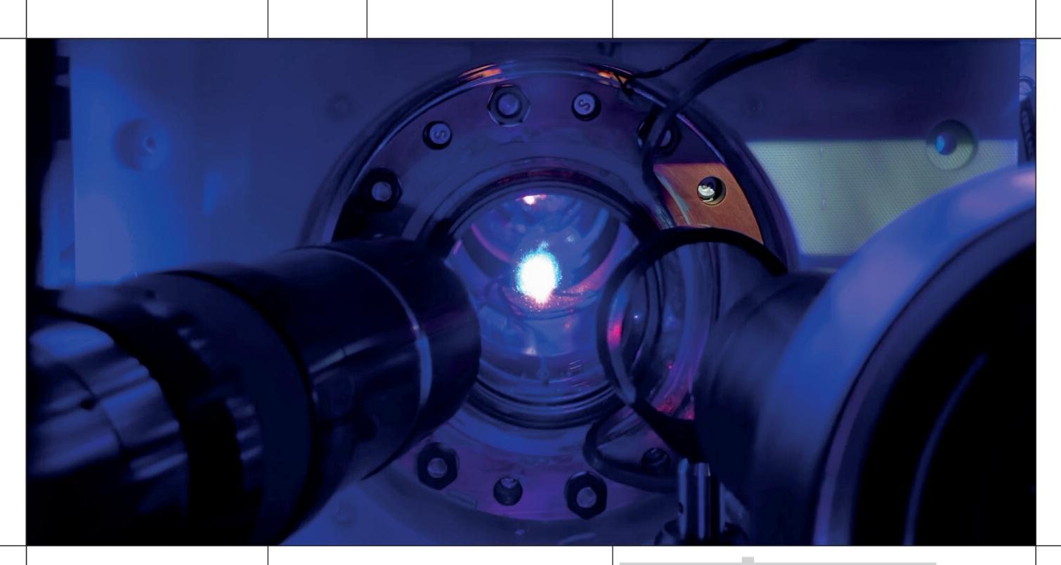
By shining an ultra-precise laser on strontium atoms, researchers have created the world's most accurate atomic clock. The laser's frequency is fine-tuned to make an electron in the strontium atom jump between its energy levels, and the clock is synchronized to this frequency. It then measures time to within a billionth of a billionth of a second.
