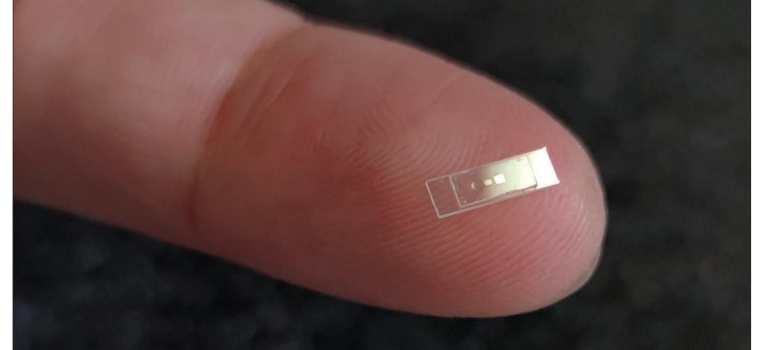
This electronic component weighs 16 micrograms—just enough to be visible to the naked eye. By cooling it, a team successfully placed it in two states simultaneously: a spring both stretched and compressed, mirroring Schrödinger's cat being both dead and alive. « Schrödinger cat states of a 16-microgram mechanical oscillator», M. Bild et al, Science (2023) Yiwen Chu team, ETH Zurich (Switzerland) @Matteo Fadel, ETH Zürich
