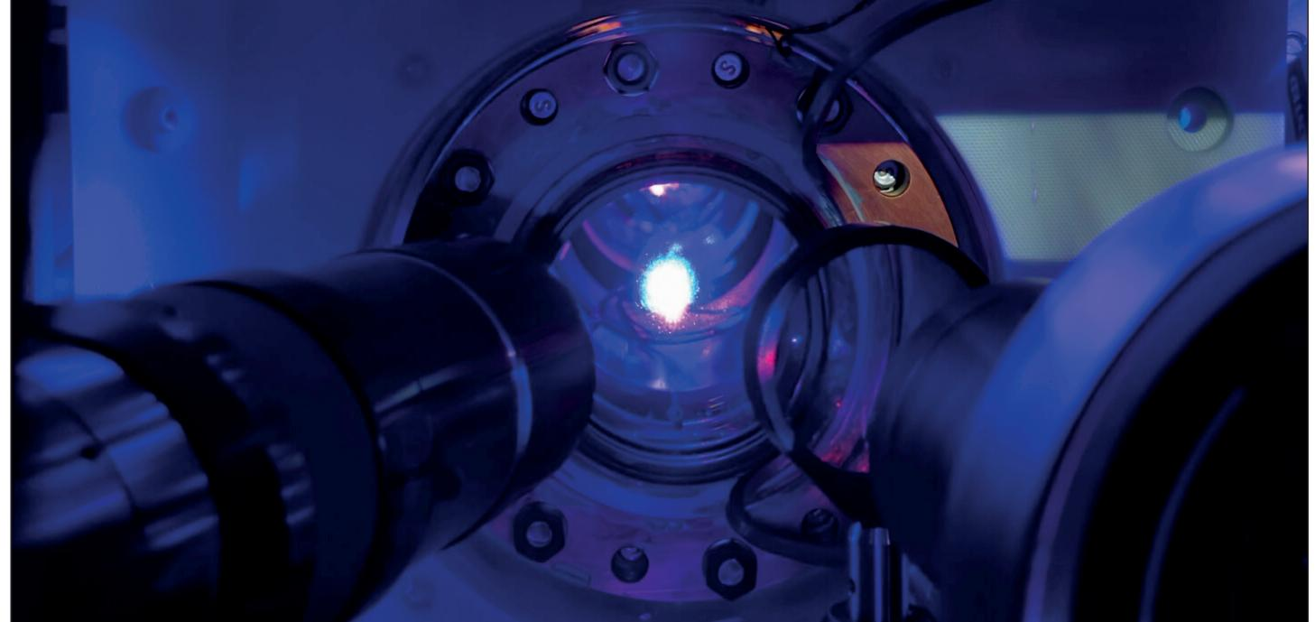
By shining an ultra-precise laser on strontium atoms, researchers have created the world's most accurate atomic clock. The laser's frequency is fine-tuned to make an electron in the strontium atom jump between its energy levels, and the clock is synchronized to this frequency. It then measures time to within a billionth of a billionth of a second. « Clock with 8× 10<sup>-19</sup> systematic uncertainty.» A. Aeppli et al., Phys. Rev. Lett. (2024) @ Kyungtae Kim, JILA
