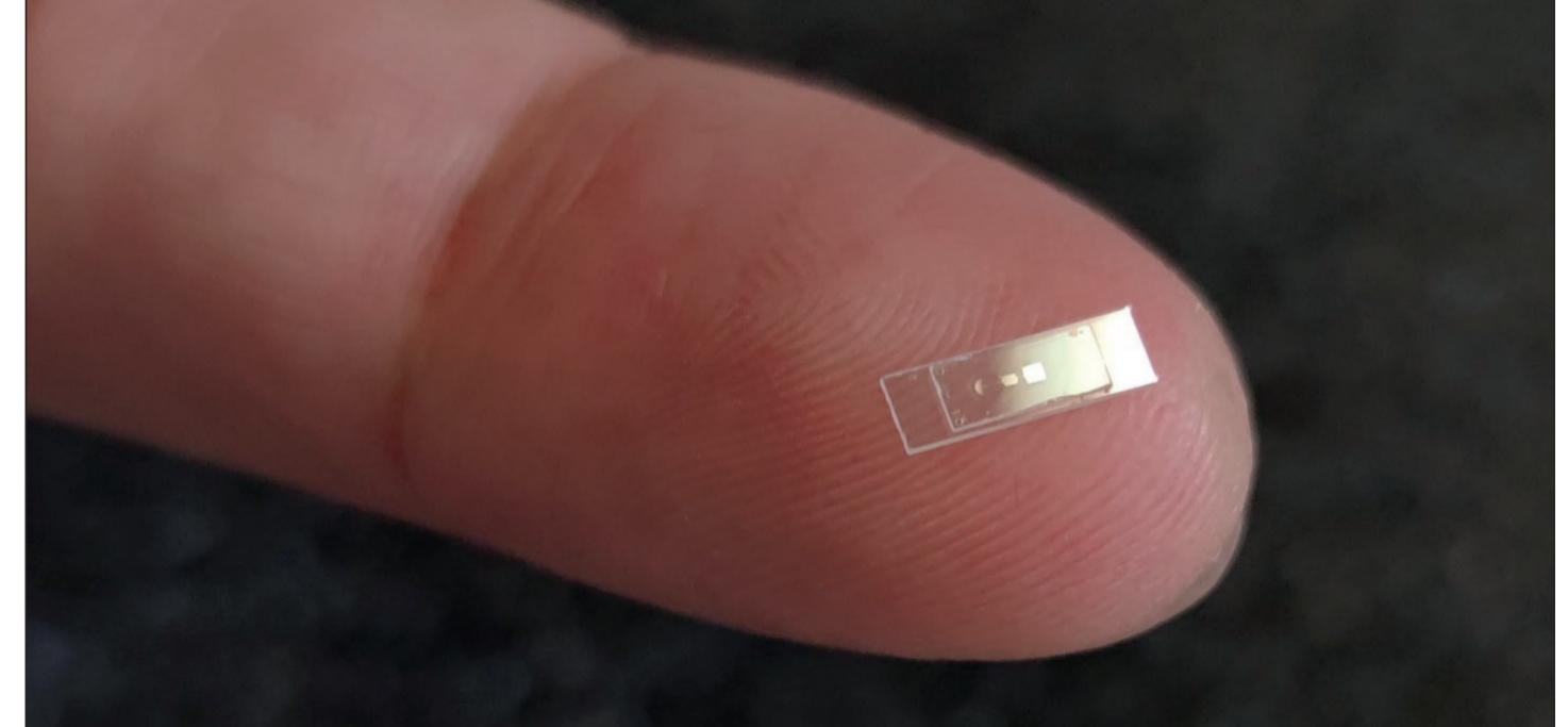
This electronic component weighs 16 micrograms—just enough to be visible to the naked eye. By cooling it, a team successfully placed it in two states simultaneously: a spring both stretched and compressed, mirroring Schrödinger's cat being both dead and alive. « Schrödinger cat states of a 16-microgram mechanical oscillator», M. Bild et al, Science (2023) @Mateo Fadel, ETH Zürich
