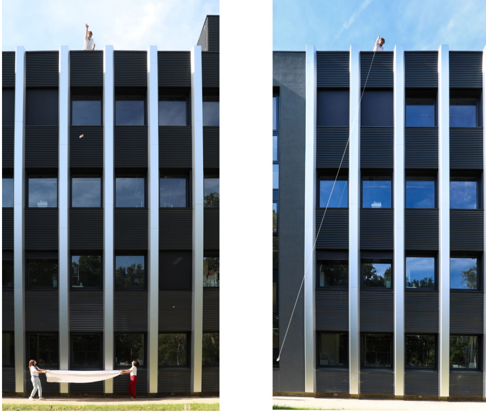
FIG. 1. Measurement of the height of the building using method #1 (free fall of a smartphone) and #13 (giant pendulum, using the smartphone's gyroscope). Results are presented in Table I.
