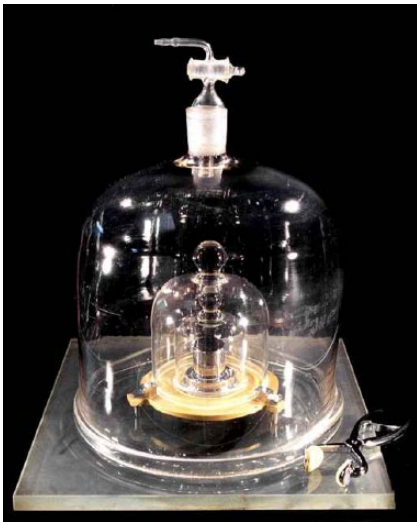
Figure 1. The International Prototype Kilogram stored at the Bureau International des Poids et Mesures in air under three bell jars
