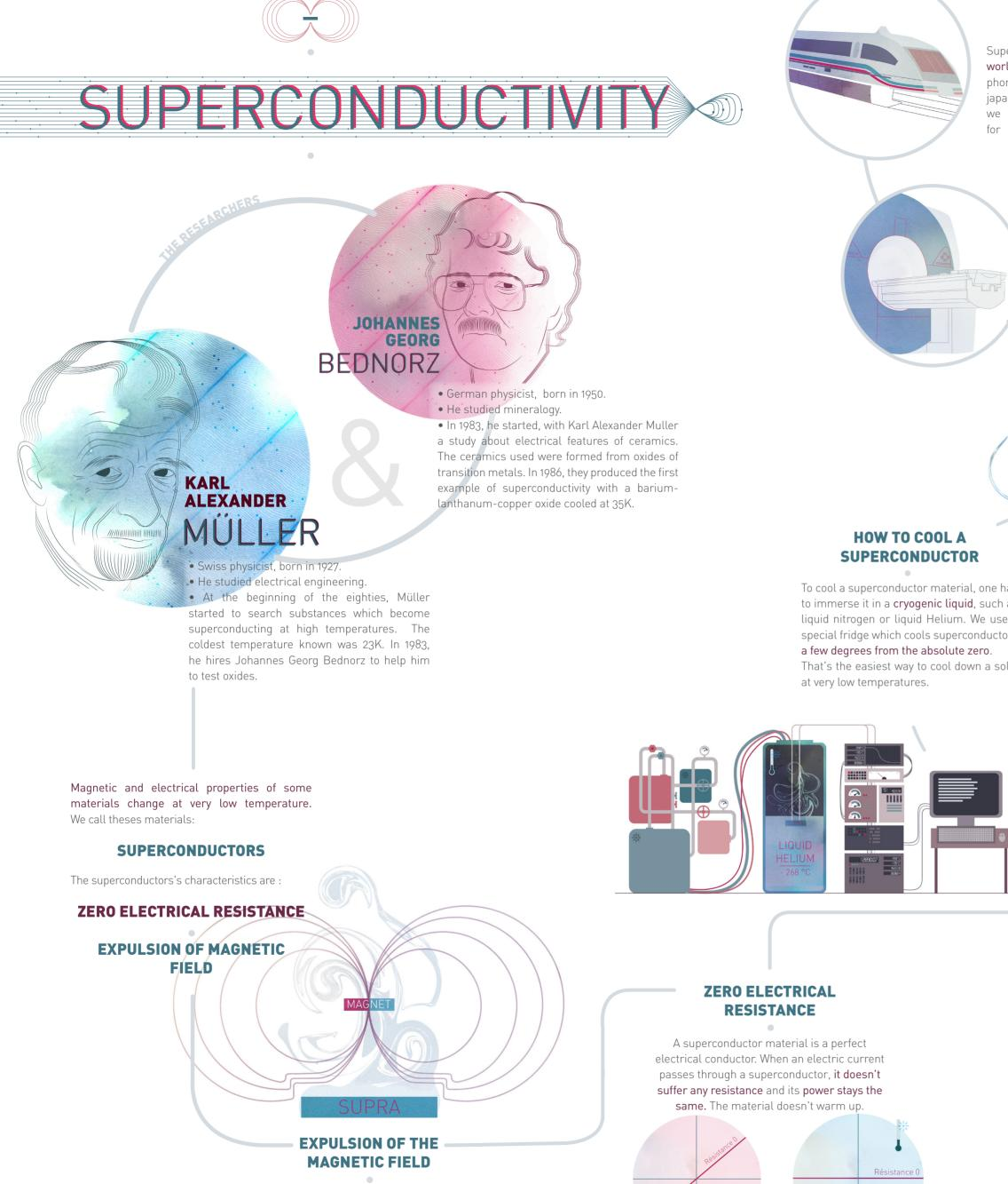
The expulsion of magnetic field enables the **levitation**.
