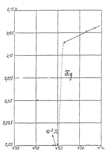
impracticable to reverse the auxiliary current as is usually done in the compensation method. The resistance of the mercury thread was then obtained from the differences between the deflections of the galvanometer placed in circuit with  $Hg_2$  and  $Hg_3$  and the compensating electromotive force, when the main current passing through the resistance was reversed. The galvanometer was calibrated for this purpose.
