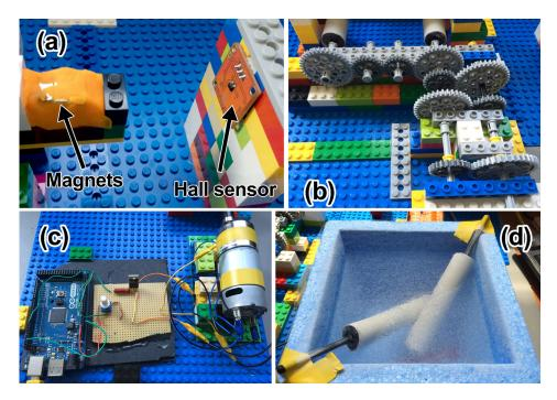
Fig. 4. (a) Detection setup; magnets are placed at the edges of the mobile plate, creating a magnetic field that is detected by the Hall sensor. (b) Zoomed view of the gearbox. (c) Zoomed view of the motor and its controller. (d) Cylinders are immersed in liquid nitrogen in preparation for a low-temperature measurement.
