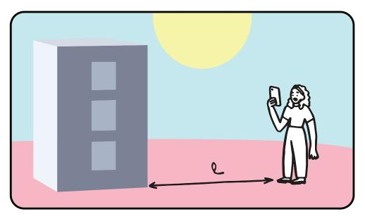
Take a picture of the building facade, at a known distance. Determine the actual size of the building image on the CCD sensor by looking at the fraction of the picture height occupied by the building.
