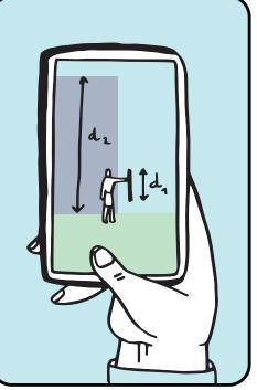
Take a picture of the facade of the building, with the bar serving as a scale. Measure the sizes of the building and the bar on the picture.
