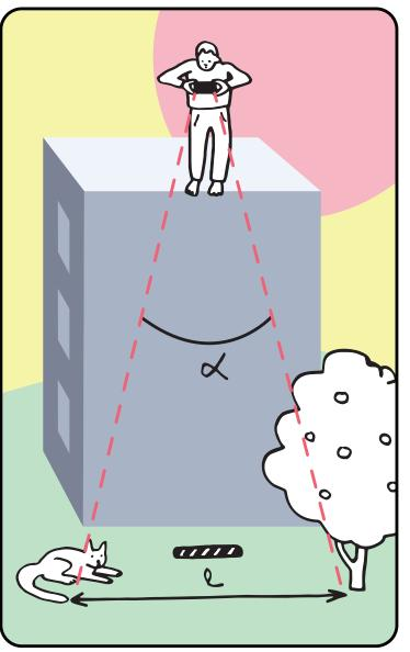
The angle of view can also be determined by taking a picture of the bar at a known distance.
