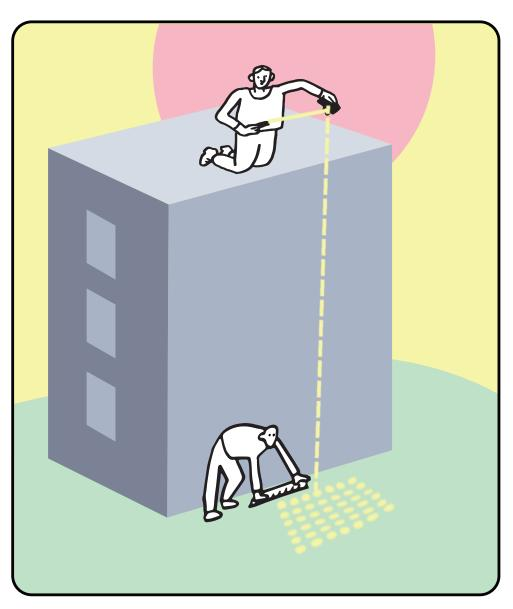
From the top of the building, illuminate the smartphone screen with the laser and project the diffraction pattern on the ground. Measure the characteristic distance of the pattern. Determine the size of the pixels by comparing their number and the size of the screen. (Some screens diffract better than others.)
