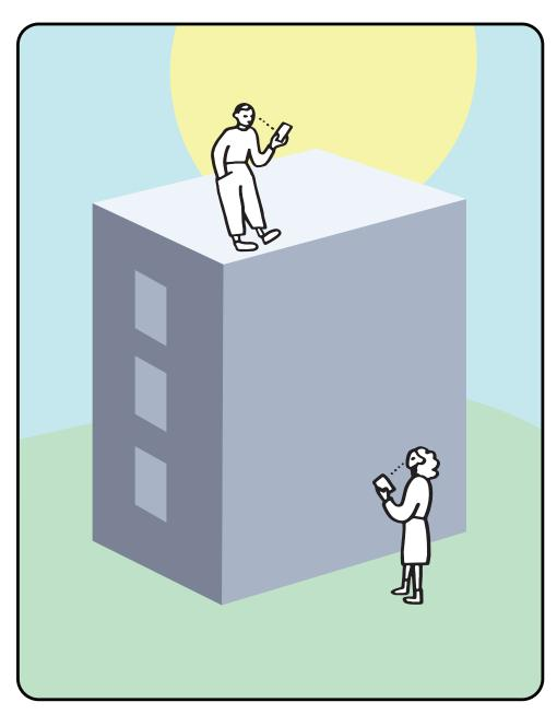
Measure the atmospheric pressure at the top and bottom of the building. The pressure variation depends directly on the height and density of air.
