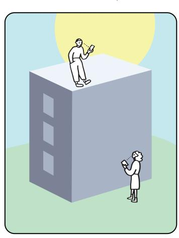
Measure the atmospheric pressure at the top and bottom of the building. The pressure variation depends directly on the height and density of air.
