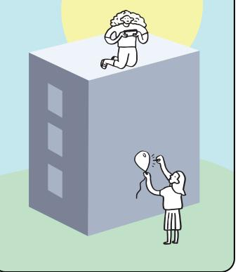
From the top of the building, film in "slow motion" the bursting of a balloon at the bottom of the building. Measure the time elapsed between the image and the sound of the exploding balloon.
