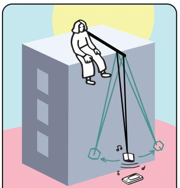
Make a giant pendulum the size of the building. Attach the speaker to the pendulum, and send a constant sound. Position the smartphone vertically, and use the variation in the amplitude of the recorded sound to determine the period.
