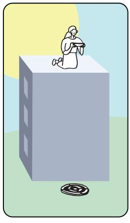
Install the target at the bottom of the building, and take a picture from the top of the building. The number of pixels representing the target in the picture varies in  $1/R^2$ , and must be calibrated before. N = number of pixels
