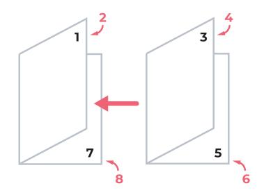
Print on two A4 sheets using both sides (select short-edge binding), then assemble the booklet by folding the sheets in two.
