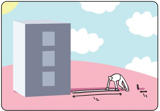
h = height of the smartphone  $I_2$  = shadow of the building,  $I_1$  = shadow of the smartphone
