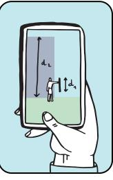
Take a picture of the facade of the building, with the bar serving as a scale. Measure the sizes of the building and the bar on the picture.
